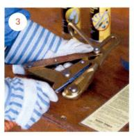
**Step 3.** Use the Klein Grip Cleaning Wire Brush to remove dirt and debris from the grip jaws (photo #3).
