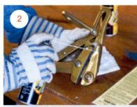
**Step 2.** Spray Klein Multi-Purpose Cleaner-Degreaser (Cat. No. 50985) on the grip jaws, all joints and moving parts (photo #2).
